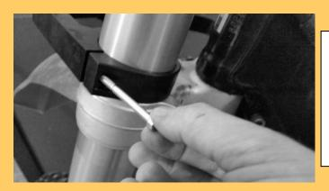
**5.** Pass the screw (1) through the hole in the flange and screw it slightly with the hand on the nut (2) that you positioned in the previous step. Do not tighten until you have the right arm mounted on the right bar.
