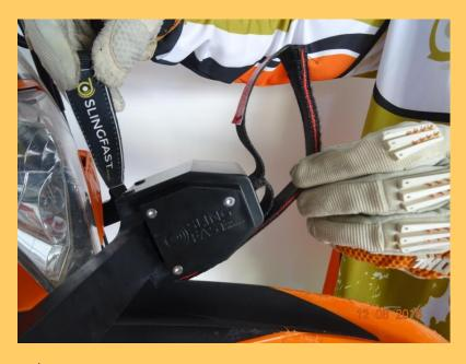
2<sup>nd</sup> Pass the fastening tape (10) through under the head (6) and pull slightly until half of traction handle (9) reaches the back of this.
