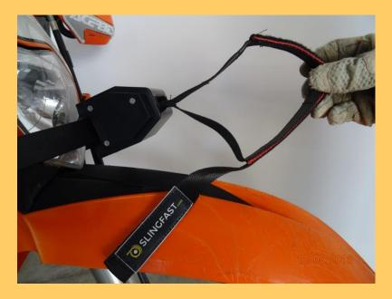
1<sup>st</sup>. Once you have stopped using the pulling strap (7), you must re-roll the handle (9) around the head (6) with the fastening tape (10).
