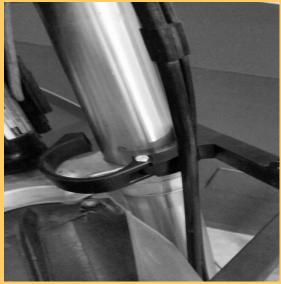
2 Start by turning the handlebar to the right to leave space between bar and chassis. Mount the left flange of SLING FAST, making it pass around the left stanchion fork, leaving all cables and wiring on the inner side of the fixing arm of SLING FAST.
