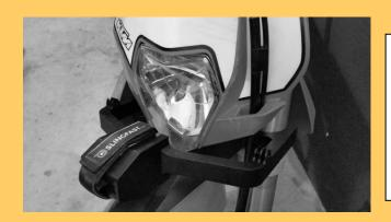
8. Reassemble the headlight, pass the cables through the cable guide of the shield or stanchion / fork leg, so that it is the same as comes standard on your motorcycle
