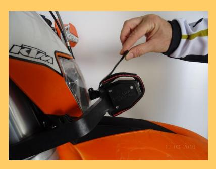
1° To start using the pulling strap (7), first you must undo the fastening tape (10) that is rolled around the head (6) pulling it to take it off the Velcro.
