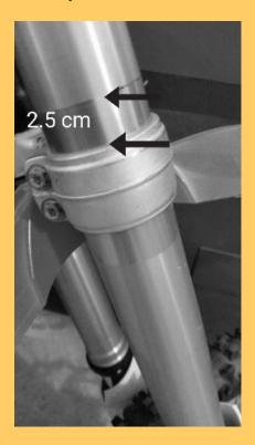
Before mounting SLING FAST you must ensure that the fork stanchions have at least 2.5 cm of space above the lower triple clamp where SLING FAST is mounted. If not, you must reposition the fork stanchion a little higher until you get an space of 2.5 mm.
