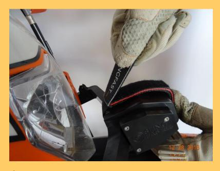
4<sup>th</sup> Now you can join the Velcro of the fixing tape with that of the traction handle (9).
