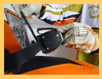
3<sup>rd</sup> Now take the upper half of the traction handle (9), which is where the Velcro is and push it down onto the top of the head (6)
