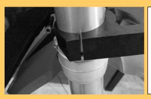
There must be a space of at least 2 mm between flange and arm, check by squeezing the flange and arm together. If your bar is less than 60 mm in diameter and there is no space between flange and arm, you must put the rubber strip (14), on the inside of the flange first to gain diameter. If one strip is not enough, mount another rubber
